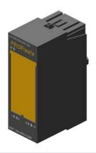
SIMATIC DP, Electronics module for ET 200S, 4 F-DO PROFIsafe, 24 V DC/2 A, 30 mm overall width, up to PL E (ISO 13849), up to SIL 3 (IEC 61508), can also be used in PROFINET configuration with IM 151-3 HF
