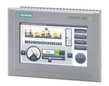
SIMATIC HMI TP700 Comfort Outdoor, Comfort Panel, Touch operation, 7" widescreen TFT display, 16 million colors, PROFINET interface, MPI/PROFIBUS DP interface, 12 MB configuration memory, Windows CE 6.0 (Microsoft Support included Security updates discontinued) configurable from WinCC Comfort V13 SP1, HSP
