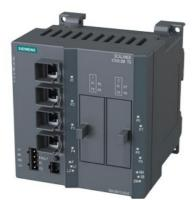
SCALANCE X308-2M TS; managed IE switch, compact; 4x 10/100/1000 Mbit/s for RJ45 ports electrical; 2x 100/1000 Mbit/s for 2-port media modules, electrical or optical; LED diagnostics; error signaling Contact; PROFINET IO device; network management; integrated redundancy manager; Office features (RSTP, VLAN, IGMP,..); C-plug in scope of delivery extended temperature range with railway approval EN 50155;
