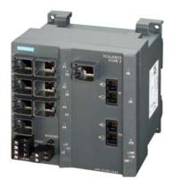
SCALANCE X308-2, managed plus IE switch, 2x 1000 Mbit/s MM SC 1x 10/100/1000 Mbit/s and 7x 10/100 Mbit/s RJ45 ports, LED diagnostics, error signaling Contact with select/set button, PROFINET IO device, network management, Integrated redundancy manager, office features (RSTP, VLAN, IGMP,..) C-plug in scope of delivery
