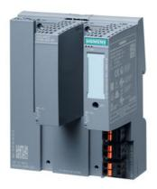
XF204-2BA IRT managed IE IRT switch, 4 x 10/100MBit/s, 2 x Bus adapter interface position, Error signaling contact, with set button, redundant 24 V DC power supply, PROFINET IO device, network management, Redundancy Manager integrated, incl. electron. manual on CD-ROM, C-plug optional
