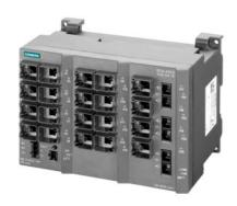
SCALANCE X320-3LDFE managed IE switch, 20x 10/100 Mbit/s RJ45 ports, 1x 100 Mbit/s SC Port MM 2x 100 Mbit/s SC Port SM LED diagnostics, error signaling Contact with select/set button, PROFINET IO device, network management, Integrated redundancy manager, office features (RSTP, VLAN, IGMP,...) C-plug in scope of delivery
