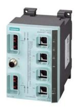
SCALANCE X204IRT PRO, managed IE IRT switch with degree of protection IP65/67, 4x 10/100 Mbit/s Push-pull RJ45 ports, error signaling contact with set button; redundant power supply; PROFINET IO device, network management, Redundancy Manager integrated, incl. electron. manual on CD-ROM, C-plug optional
