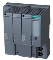
XF202-2P IRT managed IE IRT switch, 2x 10/100MBit/s RJ45 ports, 2x 100MBit/s POF SC RJ Ports, Bus adapter assembled, Error signaling contact with set button, Redundant power supply, PROFINET IO device, network management, Redundancy Manager integrated, incl. electron. manual on CD-ROM, C-plug optional
