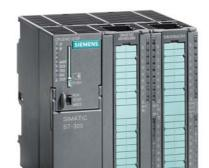
SIMATIC S7-300, CPU 314C-2 DP Compact CPU with MPI, 24 DI/16 DO, 4 AI, 2 AO, 1 Pt100, 4 high-speed counters (60 kHz), integrated DP interface, Integr. power supply 24 V DC, work memory 192 KB, Front connector (2x 40-pole) and Micro Memory Card required
