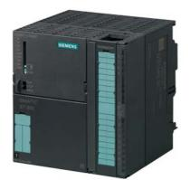
SIMATIC S7-300, CPU 315T-3 PN/DP, Central processing unit for PLC and technology tasks, 384 KB work memory, 1st interface MPI/DP 12 Mbit/s, 2nd interface DP (drive), 3rd interface Ethernet PROFINET with 2-port switch, Integr. I/O for technology, Front connector (1x 40-pole) and Micro Memory Card min. 8 MB required
