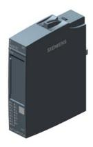
SIMATIC ET 200SP, digital input module, DI 8x 24VDC High Feature, input type 3 (IEC 61131), Sink input (PNP, active high), packaging unit: 10 pieces, suitable for BU type, A0, color code CC01, input delay: 0,05..20ms; channel diagnosis for: short circuit of sensor supply, wire break, power supply, channel failure LED
