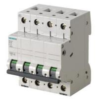
Miniature circuit breaker 400 V 6kA, 4-pole, C, 40 A
