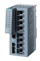
SCALANCE XC208G (E/IP) managed Layer 2 IE switch; IEC 62443-4-2 certified; 8x 10/100/1000 Mbps RJ45 ports; 1x console port; diagnostics LED; redundant power supply; temp. range -40 °C to +70 °C; mounting: DIN rail/S7 mounting rail/wall; redundancy functions; Office features (RSTP, VLAN,...); PROFINET IO device Ethernet/IP-compliant C-plug slot; Default EtherNet/IP
