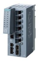
SCALANCE XC206-2SFP managed Layer 2 IE switch; IEC 62443-4-2 certified; 6x 10/100 Mbps RJ45 ports; 2x 100/1000 Mbps SFP; 1x console port; diagnostics LED; redundant power supply; temp. range -40 °C to +70 °C; mounting: DIN rail/S7 mounting rail/wall Office redundancy functions features (RSTP, VLAN,...); PROFINET IO device; Ethernet/IP-compliant; C-plug slot;
