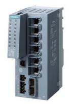
SCALANCE XC206-2SFP G managed Layer 2 IE switch; IEC 62443-4-2 certified; 6x 10/100/1000 Mbps RJ45 ports; 2x 1000 Mbps SFP; 1x console port; diagnostics LED; redundant power supply; temp. range -40 °C to +70 °C; mounting: DIN rail/S7 mounting rail/wall; redundancy functions; Office features (RSTP, VLAN,...); PROFINET IO device; Ethernet/IP-compliant; C-plug slot;
