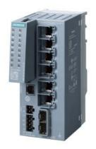
SCALANCE XC206-2SFP G (E/IP) managed Layer 2 IE switch; IEC 62443-4-2 certified; 6x 10/100/1000 Mbps RJ45 ports; 2x 1000 Mbps SFP; 1x console port; diagnostics LED; redundant power supply; temp. range -40 °C to +70 °C; mounting: DIN rail/S7 mounting rail/wall; redundancy functions; Office features (RSTP, VLAN,...); PROFINET IO device; Ethernet/IP-compliant; C-plug slot; Default EtherNet/IP
