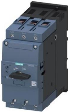
Circuit breaker size S3 for motor protection, CLASS 10 A-release 28...40 A N-release 520 A screw terminal Standard switching capacity
