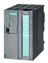
SIMATIC S7-300, FM352-5 with NPN output, High Speed Boolean Processor, for high-speed linking, 12 DI, 8 DO, 1 encoder interface for RS422 incr./SSI encoder
