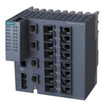
SCALANCE XC216-4C G (E/IP) managed Layer 2 IE switch; IEC 62443-4-2 certified; Full Gigabit; 12x 10/100/1000 Mbps RJ45 ports; 4x 1000 Mbps combo ports (either 1000 Mbps/ SFPs or 10/100/1000 Mbps RJ45 ports can be used); 1x console port; diagnostics LED; redundant power supply; temp. range -40 °C to +70 °C; mounting: DIN rail/S7 mounting rail/wall; redundancy functions; Office features (RSTP, VLAN,...); PROFINET IO device; Ethernet/IP-compliant; C-plug slot; Default EtherNet/IP
