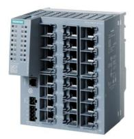
SCALANCE XC224 managed Layer 2 IE switch; IEC 62443-4-2 certified; 24x 10/100 Mbps RJ45 ports 1x console port, diagnostics LED; redundant power supply; temp. range -40 °C to +70 °C; mounting: DIN rail/S7 mounting rail/wall Office redundancy functions features (RSTP, VLAN,...); PROFINET IO device Ethernet/IP-compliant, C-plug slot;
