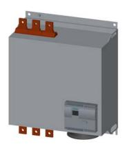
SIRIUS soft starter Values at 400 V, 40 °C standard: 970 A, 560 kW Inside-delta: 1680 A, 1000 kW 200-460 V AC, 230 V AC spring-type terminals !!! Phased-out product !!! Successor is SIRIUS 3RW5, Preferred successor type is >>3RW5556-2HA14<<
