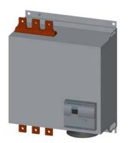
SIRIUS soft starter Values at 400 V, 40 °C standard: 970 A, 560 kW Inside-delta: 1680 A, 1000 kW 200-460 V AC, 230 V AC Screw terminals !!! Phased-out product !!! Successor is SIRIUS 3RW5, Preferred successor type is >>3RW5556-6HA14<<
