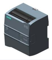
SIPLUS S7-1200 CPU 1212C DC/DC/DC for medial exposure with conformal coating based on 6ES7212-1AE40-0XB0 . compact CPU, DC/DC/DC, onboard I/O: 8 DI 24 V DC 6 DO 24 V DC 2 AI 0-10 V DC, Power supply: 20.4-28.8V DC Program/data memory 50 KB
