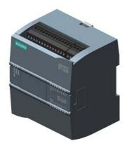
SIPLUS S7-1200 CPU 1212C AC/DC/relay for medial exposure with conformal coating based on 6ES7212-1BE40-0XB0 . compact CPU, AC/DC/relay, onboard I/O: 8 DI 24 V DC 6 DO relay 2 A 2 AI 0-10 V DC, Power supply: AC 85-264V AC @ 47-63 Hz, Program/data memory 75 KB
