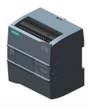
SIPLUS S7-1200 CPU 1212C DC/DC/relay -40...+70°C with conformal coating based on 6ES7212-1HE40-0XB0 . onboard "I/O: ""8 DI 24 V DC; 6 DO relay" "2 A;"" 2 AI 0-10 V DC, Power" supply: DC 20.4-28.8V DC, Program/data memory 75 KB
