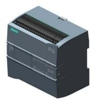
SIPLUS S7-1200 CPU 1214C AC/DC/relay -40...+70°C with conformal coating based on 6ES7214-1BG40-0XB0 . compact CPU, AC/DC/relay, onboard I/O: 14 DI 24 V DC 10 DO relay 2 A 2 AI 0-10 V DC, Power supply: AC 85-264 V AC @ 47-63 Hz, Program/data memory 100 KB
