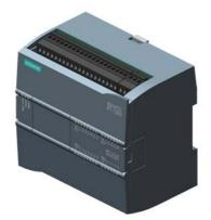
SIPLUS S7-1200 CPU 1214C AC/DC/relay for medial exposure with conformal coating based on 6ES7214-1BG40-0XB0 . compact CPU, AC/DC/relay, onboard I/O: 14 DI 24 V DC 10 DO relay 2 A 2 AI 0-10 V DC, Power supply: AC 85-264 V AC @ 47-63 Hz, Program/data memory 100 KB
