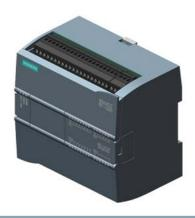
SIPLUS S7-1200 CPU 1214C DC/DC/relay -40...+70°C with conformal coating based on 6ES7214-1HG40-0XB0 . compact CPU, DC/DC/relay, onboard I/O: 14 DI 24 V DC 10 DO relay 2 A 2 AI 0-10 V DC, Power supply: DC 20.4-28.8V DC, Program/data memory 100 KB
