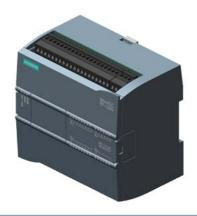
SIPLUS S7-1200 CPU 1214C DC/DC/relay for medial exposure with conformal coating based on 6ES7214-1HG40-0XB0 . compact CPU, DC/DC/relay, onboard I/O: 14 DI 24 V DC 10 DO relay 2 A 2 Al 0-10 V DC, Power supply: DC 20.4-28.8V DC, Program/data memory 100 KB
