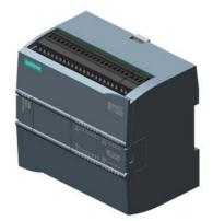
SIPLUS S7-1200 CPU 1214C DC/DC/relay -40...+60°C with conformal coating Signal board usable based on 6ES7214-1HG40-0XB0 . compact CPU, DC/DC/relay, onboard I/O: "14 DI 24 V DC; 10 DO relay 2" "A; 2 AI 0-10 V DC, Power" supply: AC 20.4-28.8V DC, Program/data memory 100 KB
