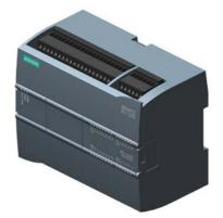
SIPLUS S7-1200 CPU 1215C DC/DC/DC with conformal coating based on 6ES7215-1AG40-0XB0 . compact CPU, DC/DC/DC, 2 PROFINET ports, onboard I/O: 14 DI 24 V DC 10 DO 24 V DC 0.5 A 2 AI 0-10 V DC, 2 AO 0-20 mA DC, Power supply: DC 20.4-28.8V DC, Program/data memory 125 KB
