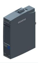
SIPLUS ET 200SP analog input module, Al 4XI 2-/4-wire Standard, -  $40...+70^{\circ}C$  with conformal coating based on 6ES7134-6GD01-0BA1 . suitable for BU type A0, A1, Color code CC03, Module diagnostics, 16 bit, +/-0.3%
