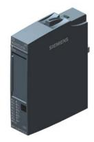
SIPLUS ET 200SP -40...+70°C start up temperature: -25°C with conformal coating based on 6ES7132-6BF00-0CA0 . digital output module, DQ 8x 24VDC/0.5A High Feature suitable for BU type A0, Color code CC02, channel diagnostics
