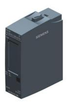
SIPLUS ET 200SP, Relay module, RQ NO 4x 120V DC..230VAC/5A ST -  $40...70^{\circ}\text{C}$  with conformal coating based on 6ES7132-6HD01-0BB1. suitable for BU type B0 or B1, Module diagnostics
