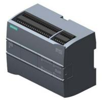
SIPLUS S7-1200 CPU 1215C AC/DC/relay -40...+70°C with conformal coating based on 6ES7215-1BG40-0XB0 . compact CPU, AC/DC/relay, 2 PROFINET Port,onboard I/O: 14 DI 24 VDC 10 DO relay 2 A 2 AI 0-10 VDC 2 AO 0-20 mA DC Power supply: 85-264V AC @ 47-63 Hz, Program/data memory 125 KB
