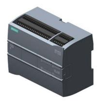
SIPLUS S7-1200 CPU 1215C AC/DC/relay for medial exposure with conformal coating based on 6ES7215-1BG40-0XB0 . compact CPU, AC/DC/relay, onboard I/O: 14 DI 24 V DC 10 DO relay 2 A 2 AI 0-10 V DC 2 AO 0-20 mA DC Power supply: 85-264V AC @ 47-63 Hz, Program/data memory 125 KB
