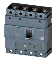
circuit breaker 3VA1 IEC frame 250 breaking capacity class S Icu=36kA @ 415V 4-pole, line protection TM240, ATAM, In=200A overload protection Ir=140A...200A short-circuit protection Ii=5...10 x In N conductor unprotected nut keeper kit
