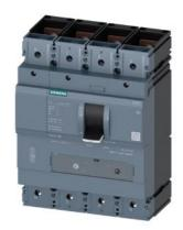
circuit breaker 3VA1 IEC frame 630 breaking capacity class S Icu=36kA @ 415V 4-pole, line protection TM240, ATAM, In=500A overload protection Ir=350A...500A short-circuit protection Ii=5...10 x In N conductor unprotected nut keeper kit
