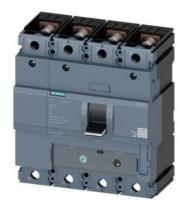
circuit breaker 3VA1 IEC frame 250 breaking capacity class M Icu=55kA @ 415V 4-pole, line protection TM240, ATAM, In=200A overload protection Ir=140A...200A short-circuit protection Ii=5...10 x In N conductor unprotected nut keeper kit
