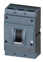
circuit breaker 3VA1 IEC frame 1000 breaking capacity class H Icu=70kA @ 415V 3-pole, starter protection TM120M, AM, In=800A without overload protection short-circuit protection Ii=6...12 x In nut keeper kit
