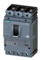
circuit breaker 3VA2 IEC frame 250 breaking capacity class M Icu=55kA @ 415V 3-pole, motor protection ETU350M, LSI, In=200A overload protection Ir=80A...200A short-circuit protection Isd=3...15 x Ir, Ii=15 x In nut keeper kit
