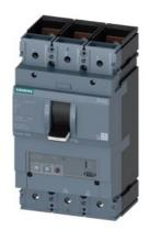
circuit breaker 3VA2 IEC frame 630 breaking capacity class M Icu=55kA @ 415V 3-pole, motor protection ETU350M, LSI, In=400A overload protection Ir=160A...400A short-circuit protection Isd=3...15 x Ir, Ii=15 x In nut keeper kit
