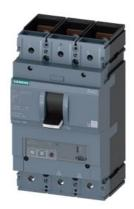
circuit breaker 3VA2 IEC frame 630 breaking capacity class M Icu=55kA @ 415V 3-pole, motor protection ETU350M, LSI, In=500A overload protection Ir=200A...500A short-circuit protection Isd=3...15 x Ir, Ii=15 x In nut keeper kit
