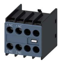
Auxiliary switch on the front, 2 NC Current path 1 NC, 1 NC for 3RH and 3RT screw terminal .1/.2, .1/.2,
