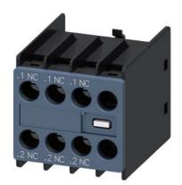
Auxiliary switch on the front, 3 NC Current path 1 NC, 1 NC, 1 NC for 3RH and 3RT screw terminal .1/.2, .1/.2, .1/.2
