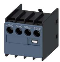
Auxiliary switch on the front, 1 NO + 1 NC Current path 1 NO, 1 NC Connection from top for 3RH and 3RT screw terminal 73/74, 81/82
