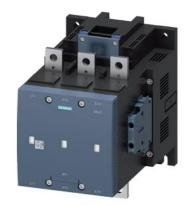
Vacuum contactor, AC-3 400 A, 200 kW / 400 V AC (50-60 Hz) / DC operation 23-26 V UC Auxiliary contacts 2 NO + 2 NC 3-pole, Size S12 Busbar connections Drive: conventional
