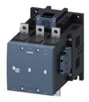
Vacuum contactor, AC-3 400 A, 200 kW / 400 V AC (50-60 Hz) / DC operation 110-127 V UC Auxiliary contacts 2 NO + 2 NC 3-pole, Size S12 Busbar connections Drive: conventional
