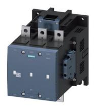
Vacuum contactor, AC-3 500 A, 250 kW / 400 V AC (50-60 Hz) / DC operation 23-26 V UC Auxiliary contacts 2 NO + 2 NC 3-pole, Size S12 Busbar connections Drive: conventional
