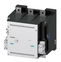
Contactor, Size 14, 3-pole, AC-3, 335kW, 400/380 V (1000 V) Auxiliary switch 44 (4NO+4NC) AC operation 110...132 V AC 50/60 Hz
